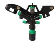
Plastic impact sprinkler with 1" female thread connection and four nozzles. Engineering plastic POM body and stainless steel spring withstands chemicals, UV radiation, and accidental impact. For field crops, vegetable and lawn by over head irrigation.
