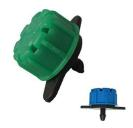
Adjustable dripper 0-100 L/H. For installation use punch 3mm. Can be placed directly onto PE pipe 16-32mm or at the end of 4/7 PVC soft hose 6mm. Ideal drip irrigation for trees, bushes and flowers.
