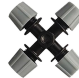
AY-1004C FOUR HEAD FOGGER- GREY PRESSURE: 1.5-3.5 BAR RADIUS: 0.9-1.1 M FLOW RATE: 30-42 L/H
