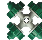
AY-1004 COLOR: GREEN OR WHITE PRESSURE: 1.5-3 BAR RADIUS: 0.7-1 M FLOW RATE: 30-35L/H
