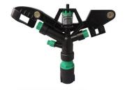
Plastic impact sprinkler with 1" female thread connection and three nozzles. Engineering plastic ABS+POM body and stainless steel spring withstands chemicals, UV radiation, and accidental impact. For field crops, vegetable and lawn by over head irrigation.
