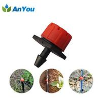
Adjustable dripper 0-70 L/H @1bar. Turn the red knob to increase or decrease the flow rate. For installation use punch 3mm. Can be placed directly onto PE pipe (Polypipe) 16mm to 32mm or at the end of 4/7 PVC soft hose 6mm. Ideal drip irrigation for dragon fruit, grape, banana, peach, trees, potted plants and flowers.
