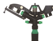
AY-5104A SIZE: 1" PRESSURE: 2-5 BAR RADIUS: 18-26M FLOW RATE: 4-6 M 3 /H
