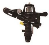
AY-5010 SIZE: 3/4" NOZZLE SIZE: 5.0*2.5MM PRESSURE: 3-5 BAR RADIUS: 13-18M
