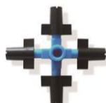
AY-1004H FOUR HEAD FOGGER PRESSURE: 2-4 BAR RADIUS: 0.6-1 M FLOW RATE: 30-40L/H
