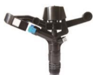
AY-5035D SIZE: 3/4" NOZZLE SIZE: 5.0*2.5MM PRESSURE: 3-5 BAR RADIUS: 13-18M
