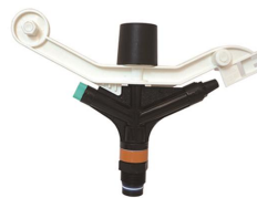
AY-5112 SIZE: 1" PRESSURE: 2-4 BAR RADIUS: 17-26 M
