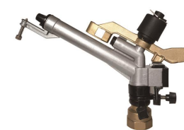
AY-1030C SIZE: 1.5" NOZZLE: 8MM/10MM/12MM/14MM/16MM PRESSURE: 3-5 BAR RADIUS: 20-30 M FLOW RATE: 6-24 M 3 /H
