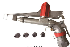
AY-1040 SIZE: 2" NOZZLE: 16MM/18MM/20MM/22MM PRESSURE: 3-5 BAR RADIUS: 28-32 M FLOW RATE: 22-36 M 3 /H
