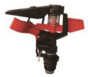
AY-5006 SIZE: 1/2" PRESSURE: 2.0-3.0 BAR RADIUS: 6-10 M 360°ADJUSTABLE
