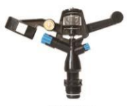
AY-5014 SIZE: 3/4" NOZZLE SIZE: 5.0*2.5MM PRESSURE: 3-5 BAR RADIUS: 5-17 M
