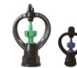
AY-1105A GREEN OR BLUE NOZZLE SIZE: 1/2" AND 3/4" PRESSURE: 1.5-3 BAR RADIUS: 3-5 M FLOW RATE: 600 L/H
