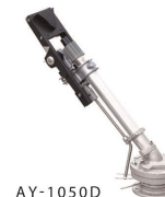
AY-1050D SIZE: 2" FLANGE PRESSURE: 3-8 BAR RADIUS: 47-80 M ANGLE: 44°
