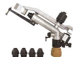
AY-1030D SIZE: 1.5" MATERIAL: ALUMINUM + BRASS PRESSURE: 1.5-5 BAR RADIUS: 20-35 M FLOW RATE: 9-32 M 3 /H
