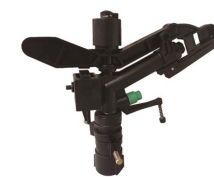
AY-5101 SIZE: 1" PRESSURE: 2-5 BAR RADIUS: 18-26M FLOW RATE: 4-6 M 3 /H
