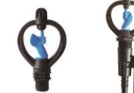
AY-1106 SIZE: 1/2" PRESSURE: 1.5-3 BAR RADIUS: 3-5 M FLOW RATE: 600 L/H
