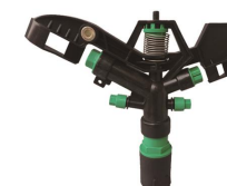
AY-5104 SIZE: 1" PRESSURE: 2-5 BAR RADIUS: 18-26M FLOW RATE: 4-6 M 3 /H
