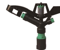
AY-5102 SIZE: 1" PRESSURE: 2-5 BAR RADIUS: 18-26M FLOW RATE: 4-6 M 3 /H
