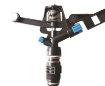
AY-5020 SIZE: 3/4" PRESSURE: 3-5 BAR RADIUS: 5-17 M FLOW RATE: 0.5-2 M 3 /H
