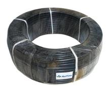
LDPE pipe for drip and sprinkler irrigation. The LDPE pipe manufactured from good quality polyethylene resins, which provide maximum resistance to UV degradation and stress cracking. Flexible and light, ideal for irrigation mainline or sub-line.
